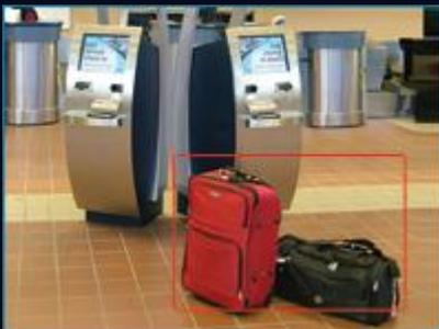
Aventura's IVA software generates an alert highlighting an abandoned object, allowing Aventura's DVR/NVRs to immediately show footage of when the item appeared, allowing the owner to be identified and correct action to be taken.
